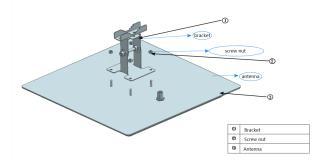
2. Fix the antenna on vertical steel frame or pillar with M8 \* 125mm screw, washer and screw nut.
